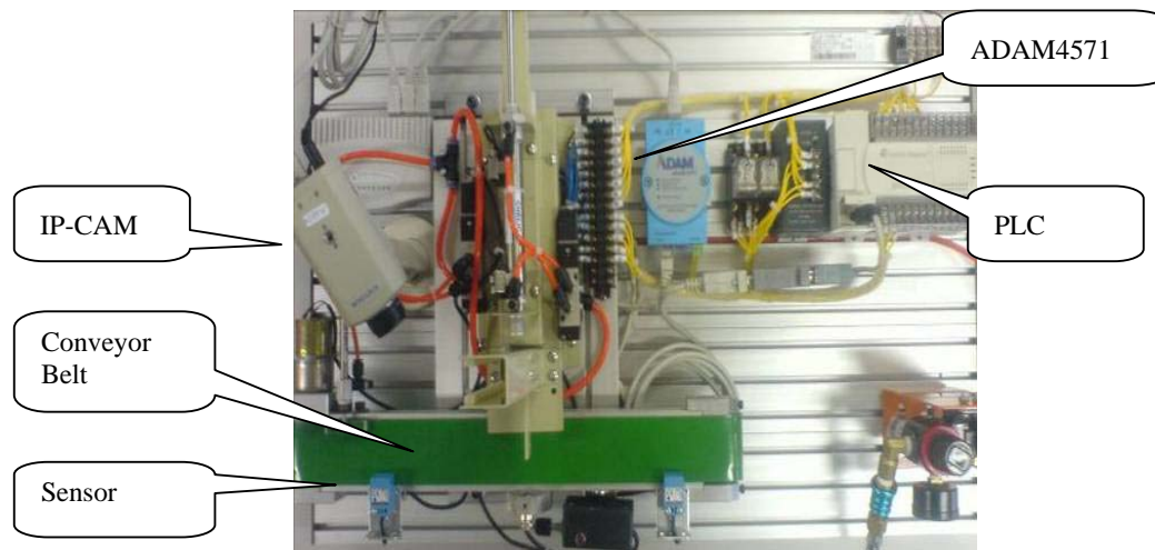
Figure. 2 Color identification module for use in the laboratory
